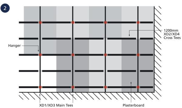
NOTE: When butt-joining on Cross Tees, it is recommended to stagger adjacent sheets for a better joint finish.
