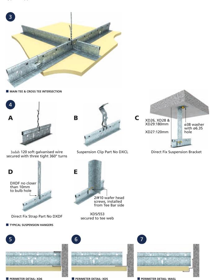
NOTE: Trim to be fixed to wall, max 600mm centres. Fixing to be relevant to wall strata (e.g. plug & screw or suitable fixings). Seismic requirements may take precedence of type and quantity of fixings.
