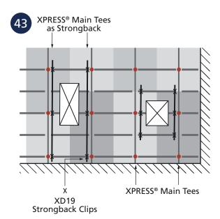
■ PLAN VIEW: PARTIAL REMOVAL OF A CROSS TEE
