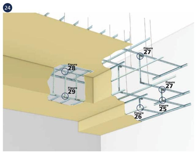
■ Judah XPRESS® DRYWALL GRID BULKHEAD/SOFFIT
