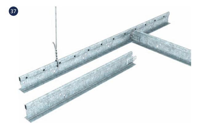
■ TYPICAL APPLICATION: OFF-MODULE GRID ARRANGEMENT (SEE ALSO FIGURE 11 ON PAGE 13)
