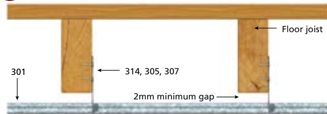
TRAFFICABLE FLOOR INSTALLATION DETAIL
