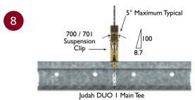
■ INSTALLING THE MAIN TEE INTO SUSPENSION CLIPS
